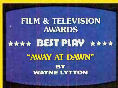
PROPORTIONAL SPACING Proportional spacing, true character overlap and variable inter-row spacing help produce captions of correct density and weight.
